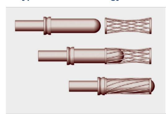
Utilized in all of our receptacle connectors, this unique design offers superior capability in every critical parameter of connector performance:
