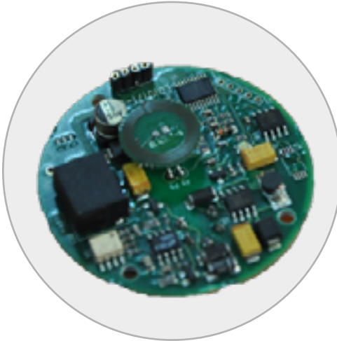
Non-contacting slip ring
