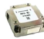
Broadband, Octave Band Circulator/ Isolator from 500MHz to 20 GHz
